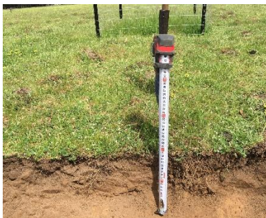
Figure 18 Photograph shows the pasture cage and soil profile cross-section where the deepest roots had reached approximately 180mm deep. The plough slipper was set to run at 280mm deep.
