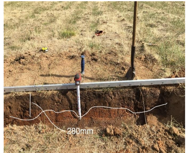
Figure 10 Soil cross-section of A&B. The white line delineates the shattered aerated zone with a maximum depth of approximately 280mm.
