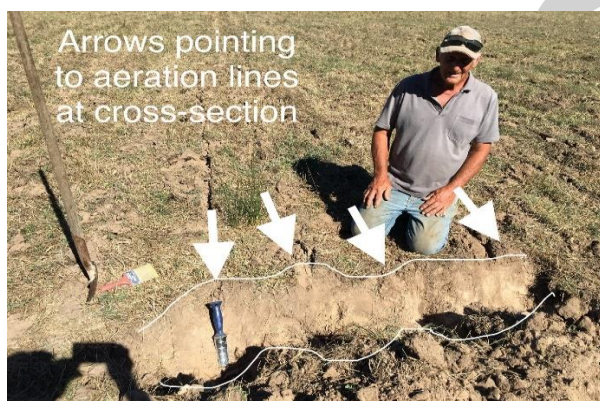
Figure 8 Shows the aeration plough depth in trial plot A&B. The trowel is 300mm long. Note the valleys and humps on the soil surface and the floor. 3 rd Feb. 2017
