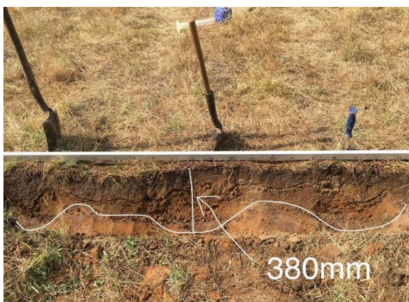
Figure 10 Soil cross-section of A. The white line delineates the shattered aeration zone. Maximum depth 380mm. Average depth 160mm.
