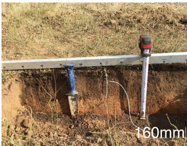
Figure 11 Soil cross-section of C. The soil depth of 160mm illustrated the old plough depth of a much earlier cultivation. Figure 12 depicts the now active topsoil layer and figure 13 the existing compaction layer.
