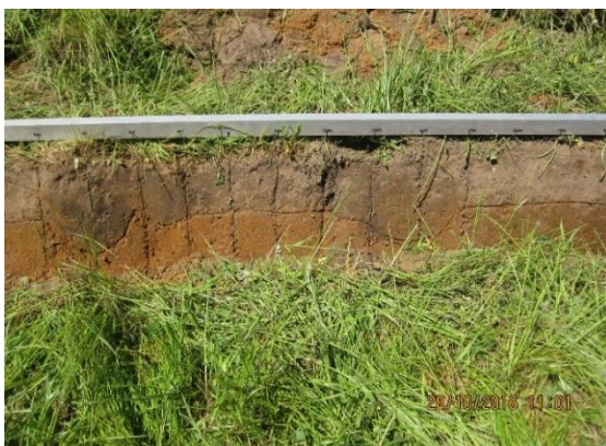
Figure 2 Shows a darkened colouration in the soil cross-section outlining the extent of the soil shattered zone that was occupied by the root curtain. The un-shattered zone has less colouration and shallower root profile.
