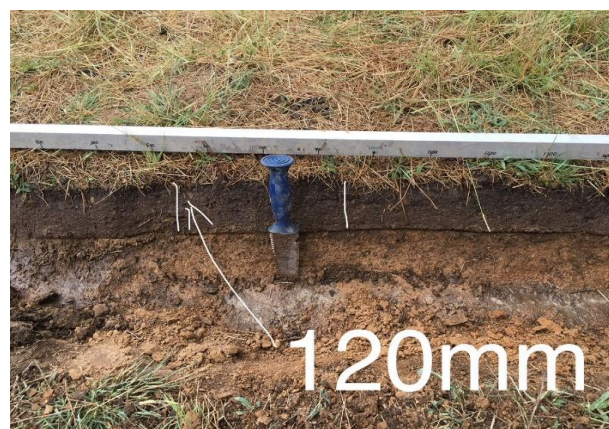
Figure 9 Soil cross-section of C. The soil depth is approximately a consistent 120mm. The trowel is 300mm long and the handle 150mm.
